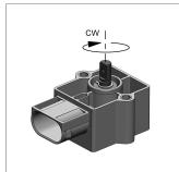
When the flattening of the shaft points towards the connector, the sensor is near the electrical center position.
