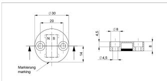
Position marker for frontal fixation with 2 cylinder head screws M4x20 (with microencapsulation, included in delivery).
